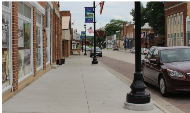
Option 2: Decorative parking treatment distinguishes the parking area from the travel lane, creating a visual separation between the street and the sidewalk (perceived safety) and enhances the streetscape.
